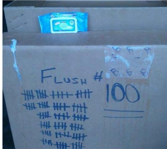
This test illustrates clearly that a wipe determined to be “flushable” by the manufacturer clearly does not break apart quickly enough to be safe to flush.
