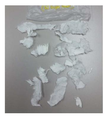
The wastewater associations believe that a product marketed as flushable should not have any accumulation in the pump. Wipes with an average power increase of less than 1% over BPD did not result in accumulation in the pump, while wipes even slightly above this value, such as the wipe pictured above, did accumulate.
