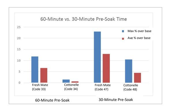
The wastewater associations believe that the 30-minute soak time is more indicative of the time that a wipe would travel through household plumbing and the municipal sewer system before reaching a pump in many wastewater collection systems. The wastewater associations therefore recommend that the soak time for pump tests be reduced to 30 minutes.
